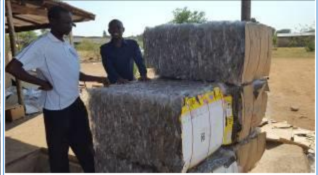
5.1.6: Mechanically compacted PET bottles. These ones for export to South Africa specifically require that the bottles be washed and caps removed
