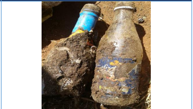
14. SOURCE OF CHARACTERISATION ERROR: GLASS HEAVILY COATED WITH ORGANICS. FULL WACS PROCESS WOULD REQUIRE WASHING, DRYING AND SUBTRACTING OF WEIGHTS TO ALLOCATE TO CORRECT WEIGHT FRACTIONS (GLASS AND ORGANICS). IN THIS BASIC CHARACTERISATION. ALL THIS WEIGHT ALLOCATED TO GLASS.
